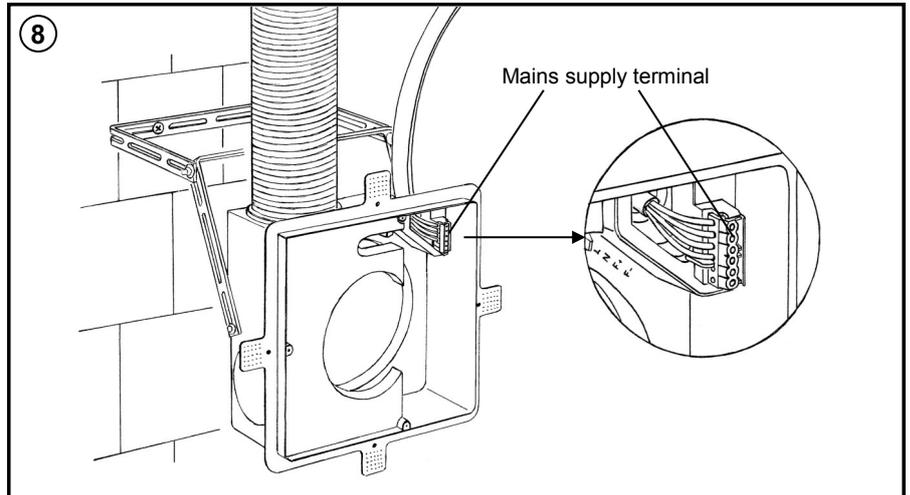
**For simple mounting of plastic housings to light-weight walls use the four mounting elements at the rim of the housing:**
