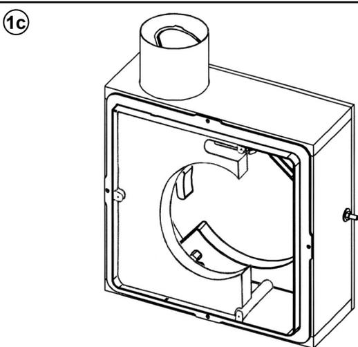
One-room fire-resistant housing with kitchen fire protection and radial exhaust opening type 3/UP-BR
