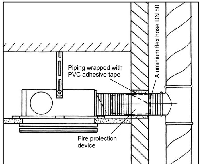
**2-Room ventilator: Duct installation**
