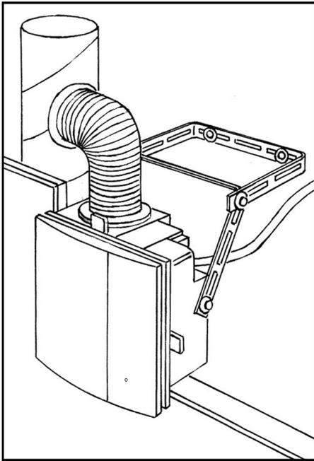
**Duct installation with kitchen fire protection**
