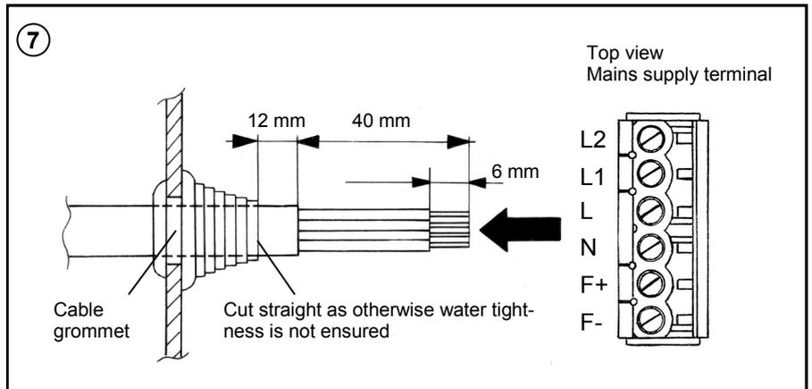
**Snap the mains supply terminal into place:**
