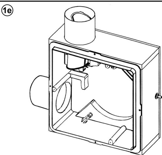
Two-room fire-resistant housing with kitchen fire protection and radial exhaust opening type 3/UP-2BR
