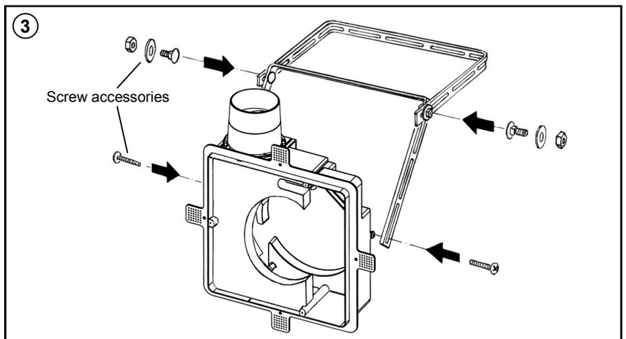
**Fix the housing to the duct wall using the mounting bracket**
