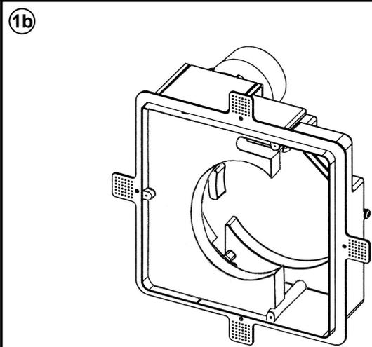
Plastic housing with axial exhaust opening type 3/UP-A
