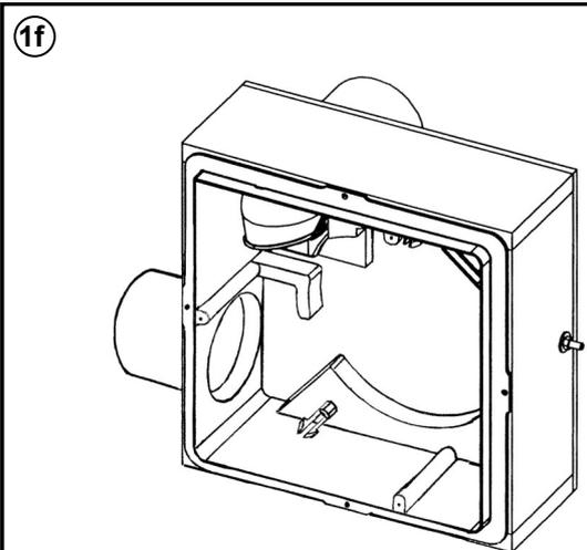
Two-room fire-resistant housing with kitchen fire protection and axial exhaust opening type 3/UP-2BA
