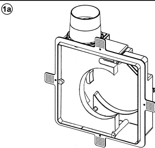
Plastic housing with radial exhaust opening type 3/UP-R
