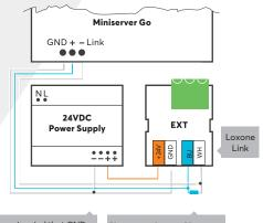
Keep in mind that GND needs to be connected to the ground of the 24V Power. Please use the 120 Ohm resistor at the last Extension which is connected to the Loxone Link.
